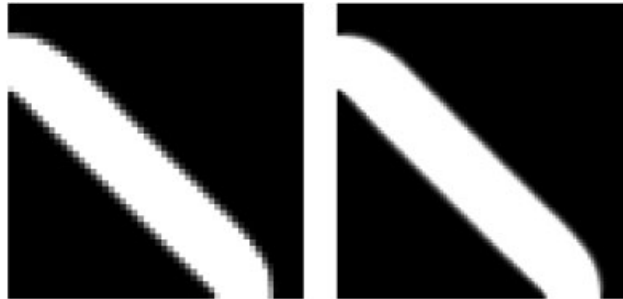
Figure 7. Optimal pipe bend on a coarse and a fine finite element mesh.
